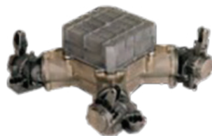
Thrust vector actuator
