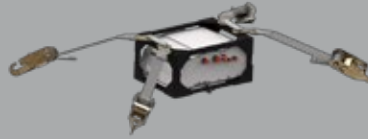
Internal Rack-mounted Subsystem (IRSS)
