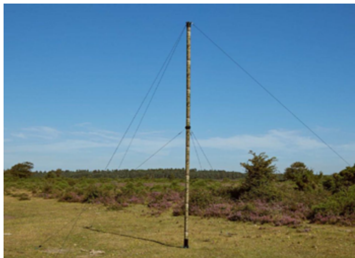
Wolf HF Broadband antenna with Rotatube mast system
