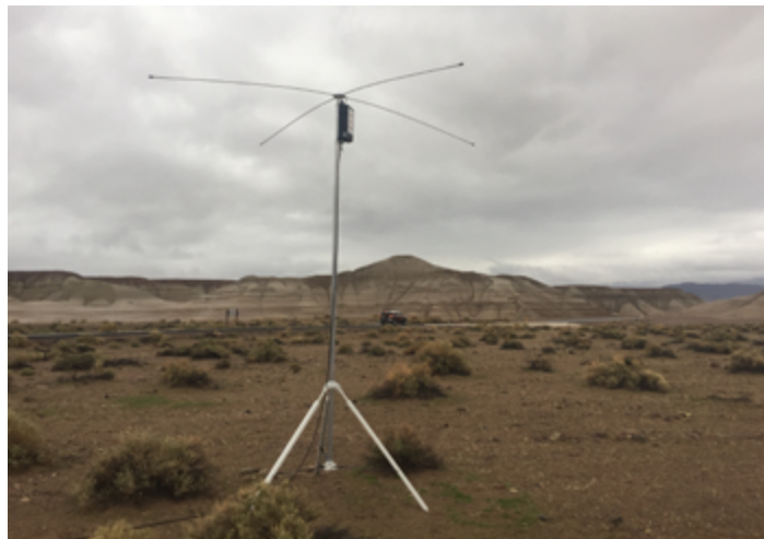
CWA-125 Omni-directional antenna with collapsible tripod mount
